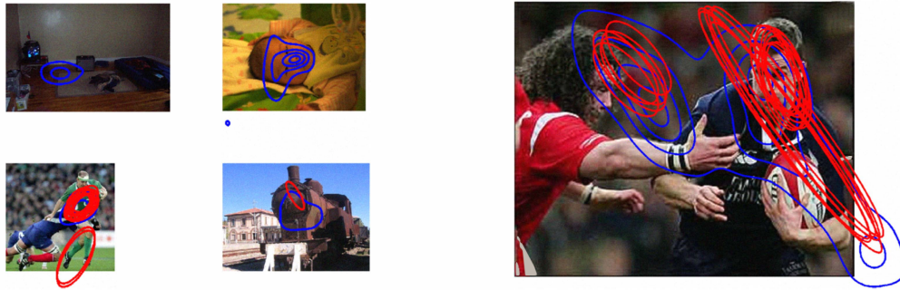
Fig. 3. Left: Demonstration of relevant region detection. The blue contours show the areas viewed by the users, while the red contours indicate the regions predicted to be most relevant for each of the users. Note how the blue contours cover regions in all images, yet the most relevant region is outside the sports image for only one user. Right: A closeup of the relevant image on one of the pages, showing how different regions of the image are chosen most relevant by different users. In both cases the relevant regions of different users have been drawn with jitter, to reveal multiple choices of the same region.
